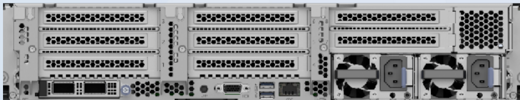
3GPU (3*double-slot or 4*single-slot GPU ) riser model
